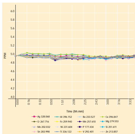
Four hour stability study for 5 mg/L S21 elements in directly aspirated kerosene, showing the stable and reliable performance of the Vista-MPX for difficult organic solvents.
